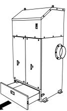
Shake dust off the filter cloth by operating the shaker handle back and forth.
