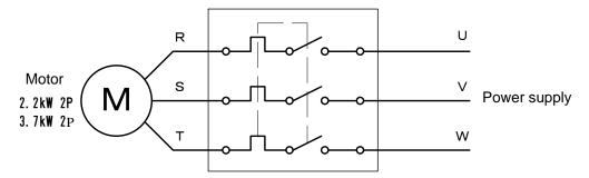
Push-button switch with protection from overload
